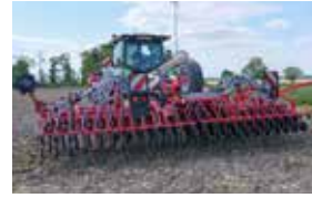
Automatically steered folding sequence of power harrow and coulters bar increase drivers comfort.
