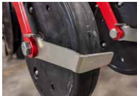
On slightly sticky soils an optional scraper is recommended.
