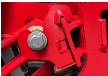
Clamped CX-II coulters to be flexible in row spacing.
