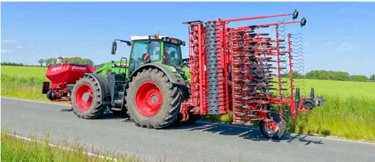
The support wheel features passive steering for safe maneuverability and allows the machine to be lifted when driving backwards. The wheel is also adjustable in height to adapt easily to different working and transport conditions. A hydraulic cylinder with an accumulator absorbs shocks and prevents bouncing.
