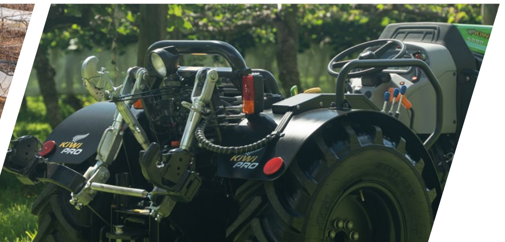
> New hydraulic control arrangement.
