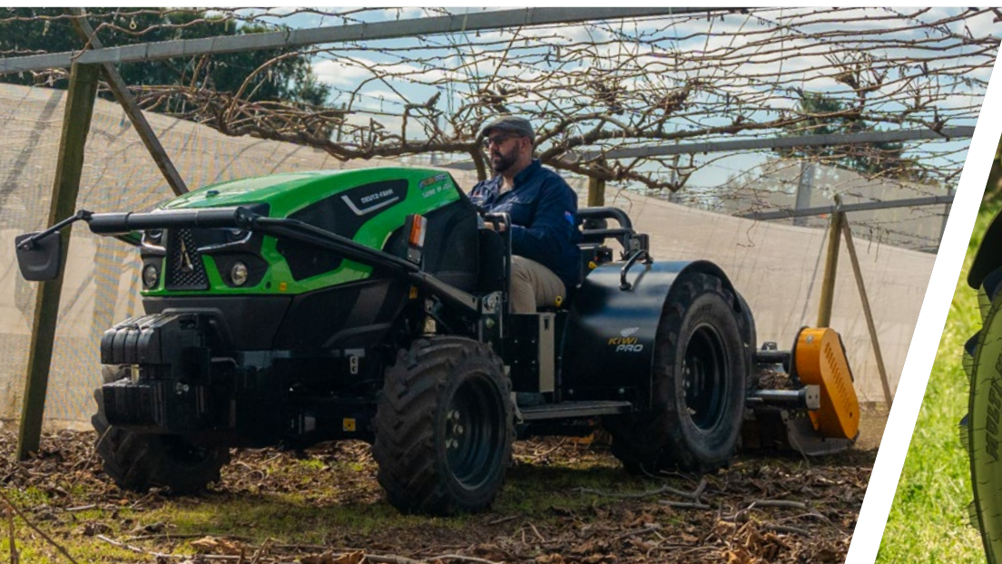
> Rugged and durable both in the field and on the road the front axle also offers a 60° steering angle.
