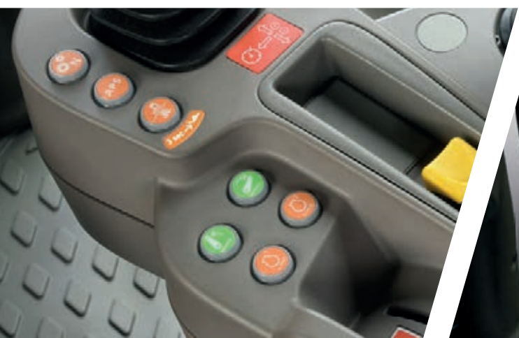
> Transport, Field, Creeper driving modes selection.
