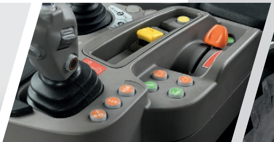
> Electronic hand throttle with 2 engine memory speeds.
